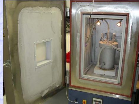
sample container within freezing chamber
